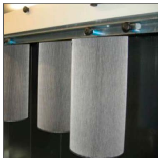
Cartucce in poliestere alluminato Aluminized polyester cartridges
